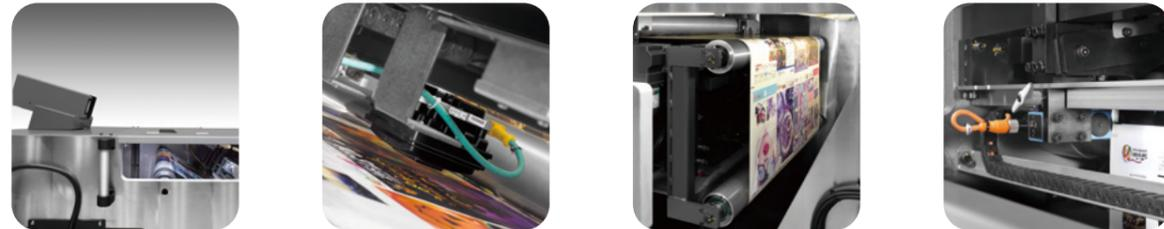
1 Density monitoring camera    2 Register monitoring camera    3 Web guide    4 Cutoff monitoring camera
